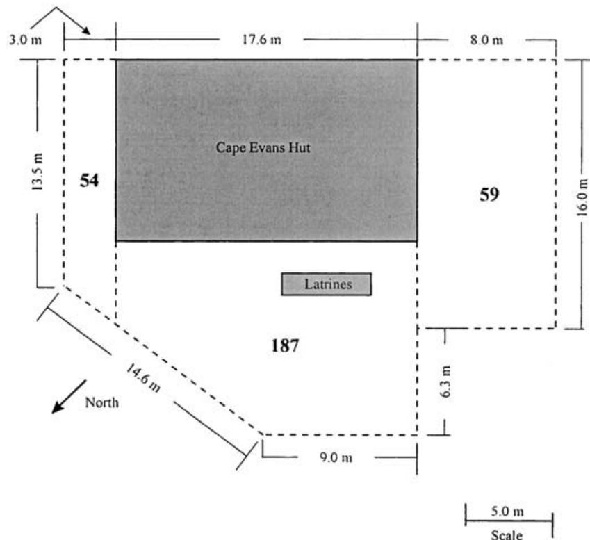
Fig. 4. Diagram of the area around Cape Evans hut with amounts of asbestos fragments greater than  $1 \text{ cm}^2$  observed on the ground surface. Numbers in bold represent the mean number of asbestos fragments determined within three snow-free areas around the hut.
