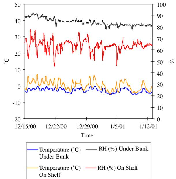
**Fig. 8.** A comparison of temperature and RH from two data loggers with different vertical positions in Cape Royds hut.
