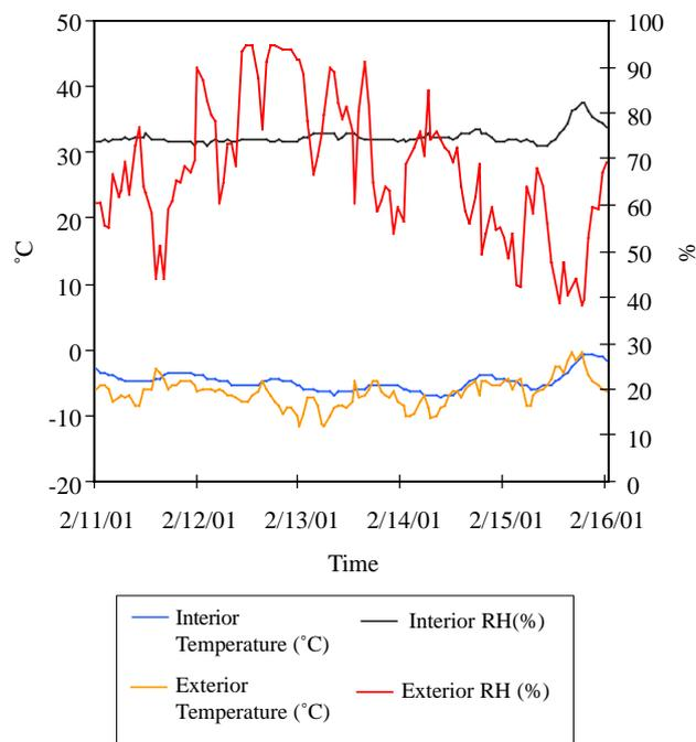
Fig. 11. Temperature and relative humidity of the exterior and interior environments at Cape Evans hut. Twenty-eight visitors entered the hut on 2/13/01. No visitors entered the hut 2 days before or after.
