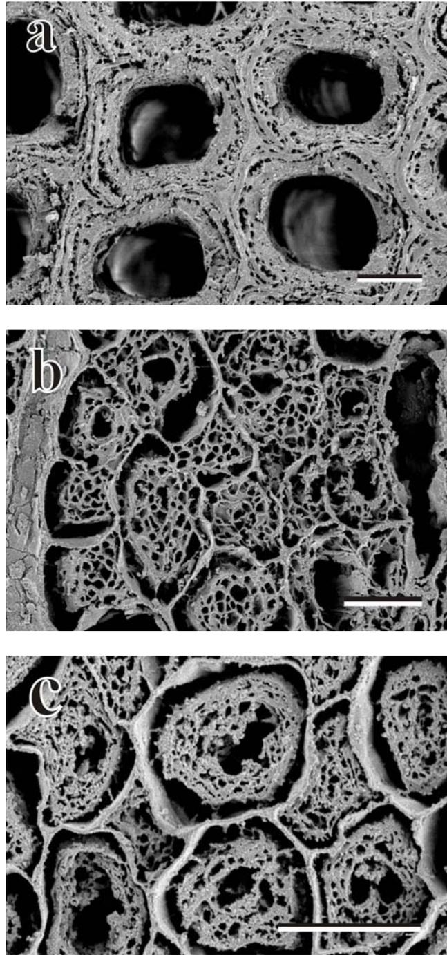
[FIGURE 6] Transverse sections of degraded *Pinus* sp. [a], *Quercus* sp. [b] and *Ulmus* sp. [c] recovered from the *Tektaş Burnu* shipwreck. All wood samples show degradation caused by erosion, tunneling and scavenging bacteria and environmental influences. Bars = 10 µm.
