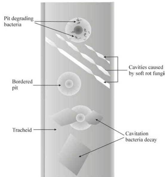
[FIGURE 1] Diagrammatic representation of a transverse view of a wood cell and cell wall layers with several types of wood degrading bacteria. [FIGURE 2] Longitudinal view of a wood cell, with degradation caused by cavitation and pit degrading bacteria and soft rot fungi.
