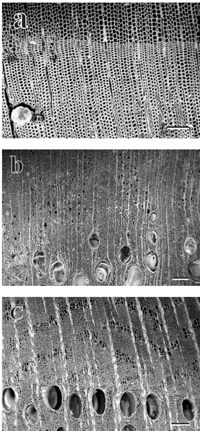
[FIGURE 5] Transverse sections of *Pinus* sp. [a], *Quercus* sp. [b] and *Ulmus* sp. [c] recovered from the *Tektaş Burnu* shipwreck. Bars = 200  $\mu$ m.
