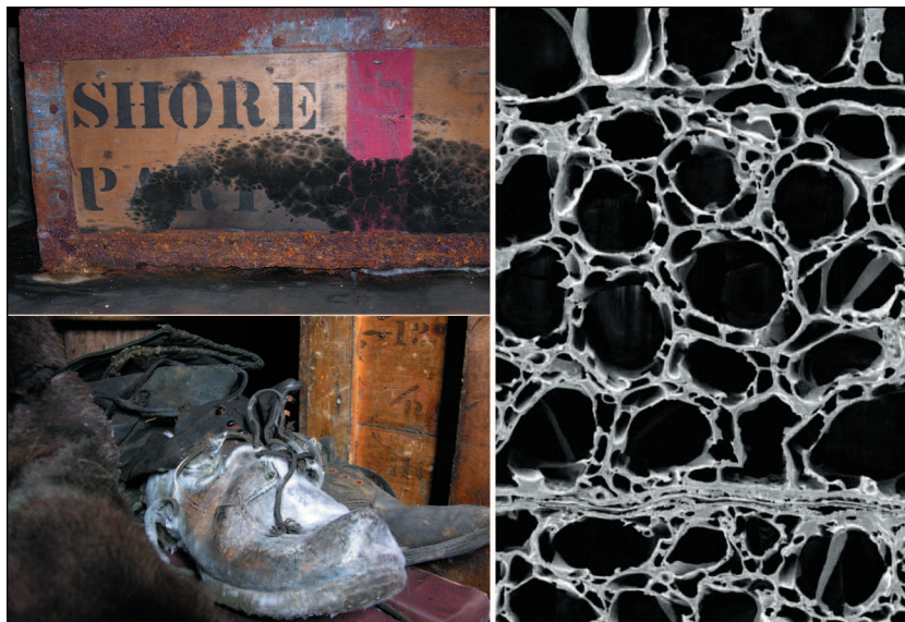
Biodeterioration of cultural properties from Scott's Cape Evans hut. Left: mold growing on a historic crate (top) and explorer's boot (bottom). Right: Wood decay cross section from Shackleton's Cape Royds hut showing extensive cavities in wood cell walls. (Figure by Benjamin Held, University of Minnesota).
