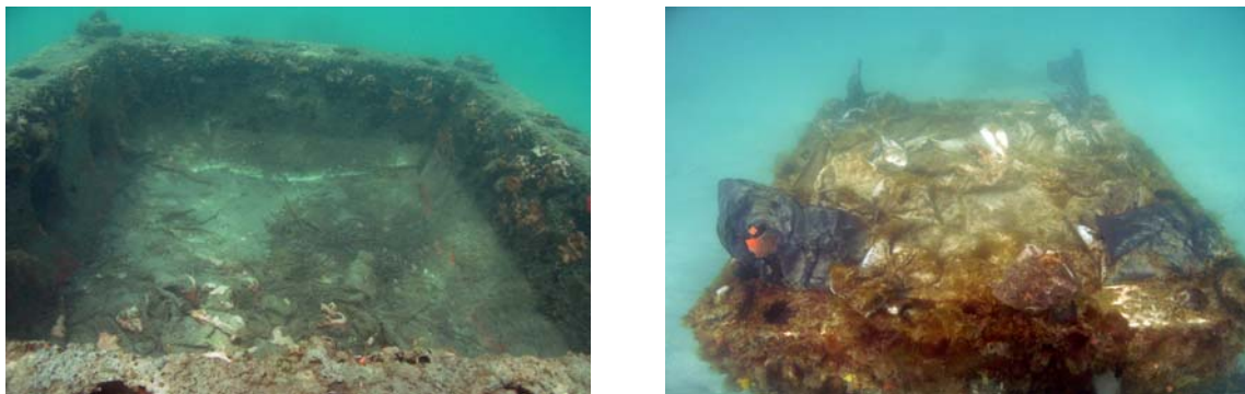
Figure 18. The test square after a) one year with significant sediment loss and b) three months after refilling.
