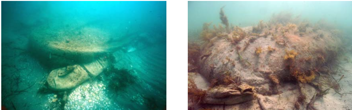
Figure 16. Sediment accretion under the shade cloth mat deployed off site after a) three months and b) two years.
