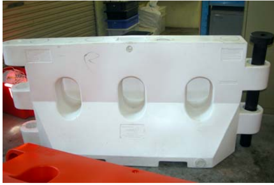
Figure 3. a) Crash barrier unit with enclosed holes; b) Example of assembled crash barrier units prior to experimental deployment.
