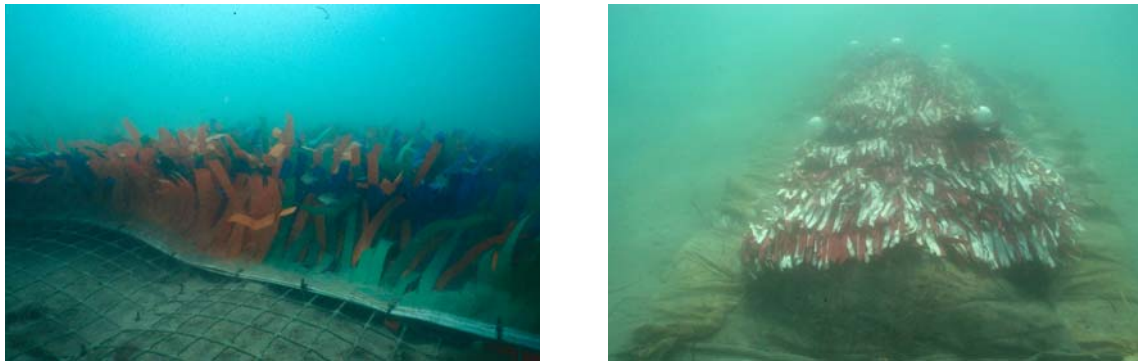
Figure 5. a) Artificial seagrass mat in-situ; b) Artificial seagrass attached to shade cloth mat in-situ.
