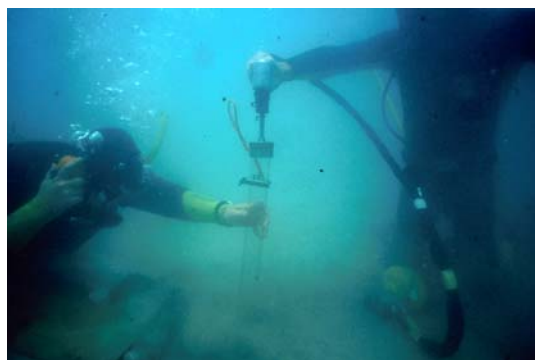
Figure 6. Polycarbonate sediment corer with hammer chisel and attachment.
