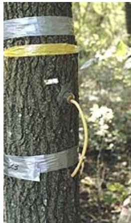
Fig. 5. The apparatus adapted from Sharon and Shigo (14) used to cover inoculated holes. Rubber tubing filled with sterile cotton was substituted for a test tube. The apparatus enables oxygen to circulate but prevents contamination.
