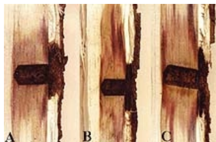
Fig. 6 Red stain in boxelder 12 wks after inoculation with (A) F. acuminatum , (B) H. tessulatus , and (C) control.
