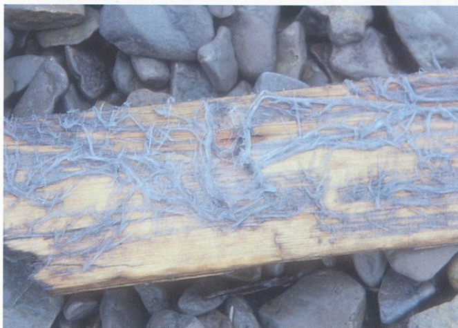
Defibration of wood surfaces was found on some woods at Beechey Island and at Fort Conger. Salt accumulation is responsible for causing a chemical attack on wood that results in the separation and detachment of wood cells. Loose surface wood fibers are eroded off exposing new cells to the corrosive action of the salts. Both photos: R.A. Blanchette
