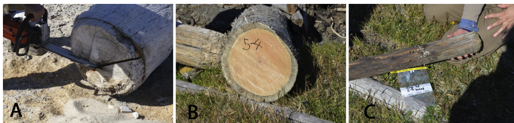
Fig. 2. Sampling of Arctic driftwood for fungal investigations. (A) Sampling with the chainsaw to obtain discs with a full radius. (B) Wood affected by blue stain fungi showing dark staining in the sapwood. (C) Samples were labeled and packed in sterile plastic bags directly after cutting.
