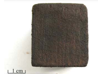
Figure 17 Cross-section of MG sample showing homogenous appearance.
