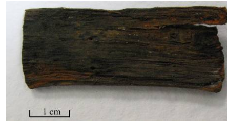
Figure 19. Sample 30d split due to air drying.
