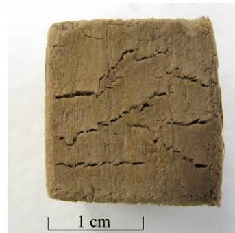
Figure 20. Cracking exhibited by MD sample 89.
