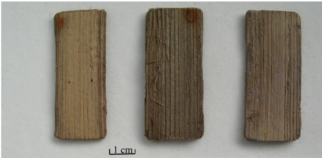
Figure 50. Treated MD planks. Left to right- air-dried sample 48b, freeze-dried sample 48c, supercritical-dried sample 48a.
