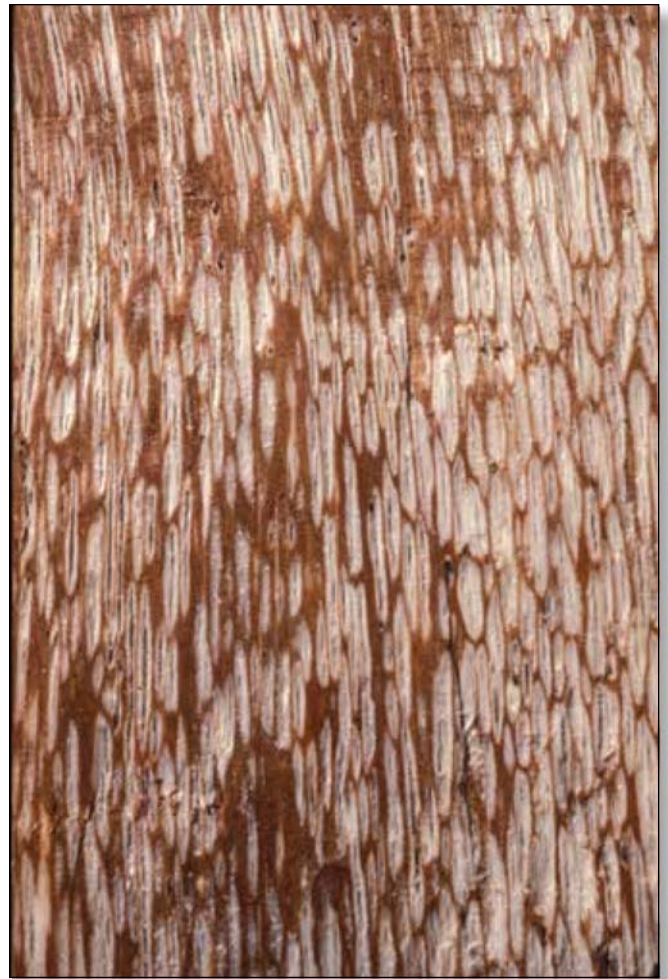
Figure 5. White pocket rot fungi are another type of white rot. Behind the fruiting bodies of fungi such as Porodaedalea pini (previously called Phellinus pini ), a fungus that attacks conifers (upper left) selective degradation of lignin and hemicellulose occurs in the wood while cellulose is left relatively untouched. Spindle-shaped pockets of white cellulose occur in the wood (upper right and page 15 photo). A scanning electron micrograph of a cross section of delignified wood shows the cellulose rich parts of the walls remaining and the area between cells (the middle lamella where most of the lignin is concentrated) removed. It is an extraordinary ability to degrade lignin, one of the most recalcitrant natural substrates known, while not removing cellulose.
