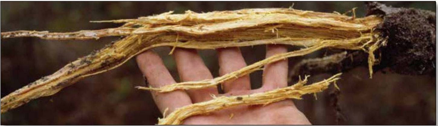
Figure 9. Some white rot fungi such as Heterobasidion , a serious root rot of conifers, produce decay that is stringy (top photo). The fungus causes a simultaneous attack on all cell wall components that leaves many eroded areas throughout the wood. The weakened wood shreds and separates into a stringy mass as it is pulled apart. Under certain conditions, some Heterobasidion species are more selective in their degradative attack causing delignification. This results in large amounts of white cellulose remaining in the decayed wood (middle photo). Although somewhat rare to find, extensive delignification can occur. In southern beech trees located in the coastal rainforests of Chile, a decay called "palo podrido" can be found (bottom photo). Entire logs can be delignified by some white rot fungi that selectively remove lignin and leave massive amounts of cellulose in the residual decay wood.
