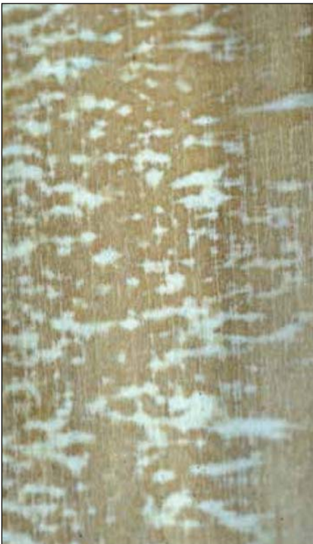
Figure 8. Ischnoderma resinorum , the benzoin bracket, (top of page) produces a decay that mimics white pocket rot; instead of pockets of delignified cells containing cellulose, this simultaneous white rotter has degraded voids in wood that fill with fungal mycelia (photo on left). A scanning electron micrograph shows one of the white zones (photo on right). The cell walls are degraded and voids are filled with remnants of the woody cell walls and masses of mycelium.
