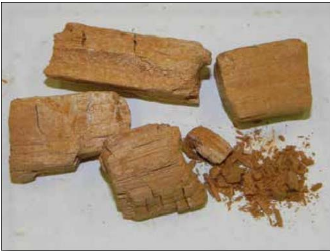
Figure 2. Brown rot fungi are cellulose degraders; when the cellulose is degraded and depolymerized the wood loses its strength properties. Decayed wood is rich in lignin giving the rot its brown color (left photo). Although brown-rotted wood may appear intact, without cellulose the wood breaks into fragments easily. A scanning electron micrograph (right photo) shows the fragile cell walls of brown rot that have crumbled into minute pieces with just a slight touch.
